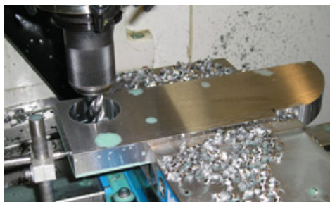
Figure 7. Machining an IIW block in a computer numerically controlled mill.
