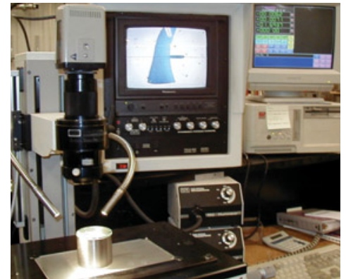
Figure 6. Video measurement system measuring the cross-section of a cast replica of an EDM notch.
