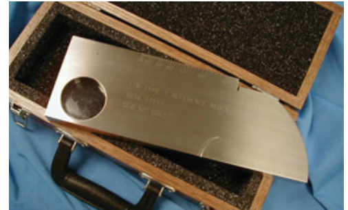
Figure 1. ASTM E164 IIW-Type 1 test block in 1018 Steel.
