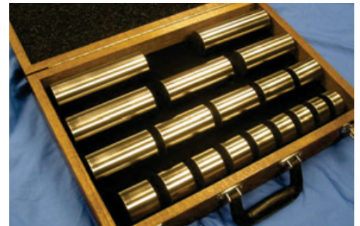
Figure 2. ASTM E428 distance amplitude set of 19 flat bottom hole (FBH) blocks in 4340 steel.
